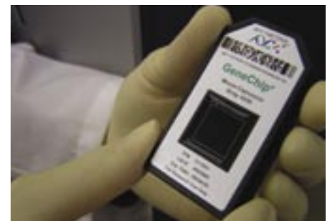
The Affymetrix machine (top) was recently installed and can analyse 500,000 individual variations from a sample of human DNA on a gene chip (bottom)
